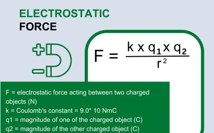
r = distance between the center of the two charges (m)
